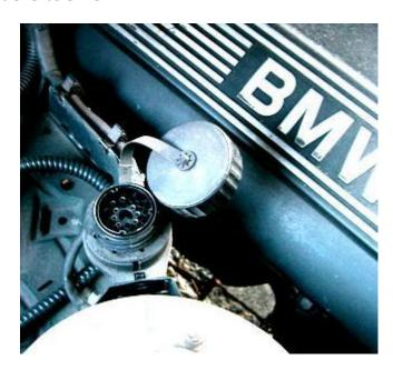
The picture shows a typical view on the 20pin socket after the dust cap got twisted off.
